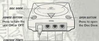
Use these ports to connect the Sega Dreamcast™ controller or other peripheral equipment. From left to right are Control Port A, Control Port B, Control Port C, and Control Port D. Tomb Raider: The Last Revetation uses Control Port A.
